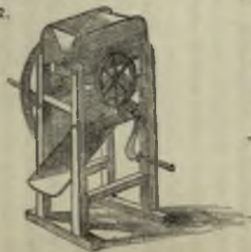
Fig. 1.—MACHINE FOR CRUSHING OATS OR GRINDING BARLEY.
